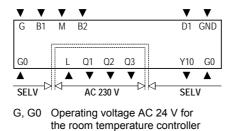
Operating voltage AC 230 V for the L fan speeds
