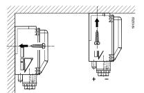
If the pressure connection nipples point upward or are at a lower level than the air duct probes, condensation can collect inside the sensor, causing damage to the device.
