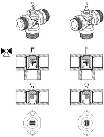
**Flow setting** At the actuator the end stop clip has to be removed. This in order to get the angle of rotation of 90°, which is needed for the change-over functionality.
