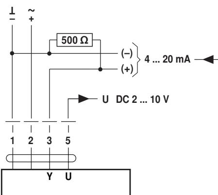
The 500  $\Omega$ -resistor converts the 4 ... 20 mA current signal to a voltage signal DC 2 ... 10 V. Operating range adjusted on DC 2...10 V
