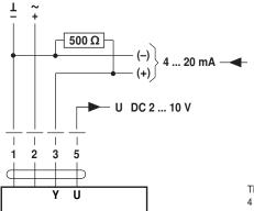
The 500  $\Omega$  resistor converts the 4 ... 20 mA current signal to a voltage signal DC 2 ... 10 V
