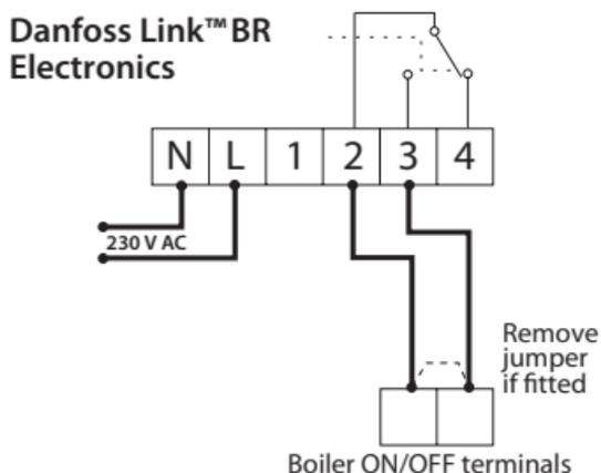
*Note: Refer to boiler manufacturer's manual for wiring connections to the boiler.*
