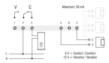
Figure 5: Dry contact to thermostat
