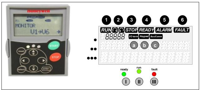
Figure 7-1. The control keypad and drive status indications
