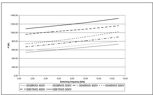
Figure 5-9. Power loss as function of switching frequency; 0038...0061NX5
