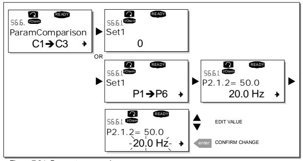
Figure 7-21. Parameter comparison
