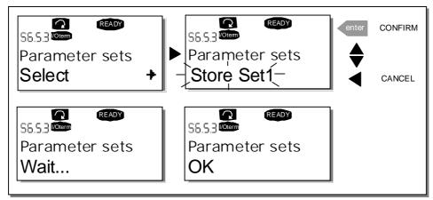
Figure 7-20. Storing and loading of parameter sets
