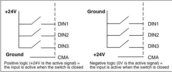
Figure 6-18. Positive/Negative logic
