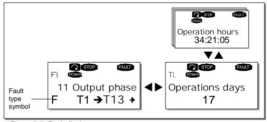
Figure 7-7. Fault display
