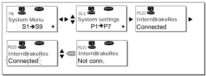
Figure 7-13. Internal brake resistor connection
