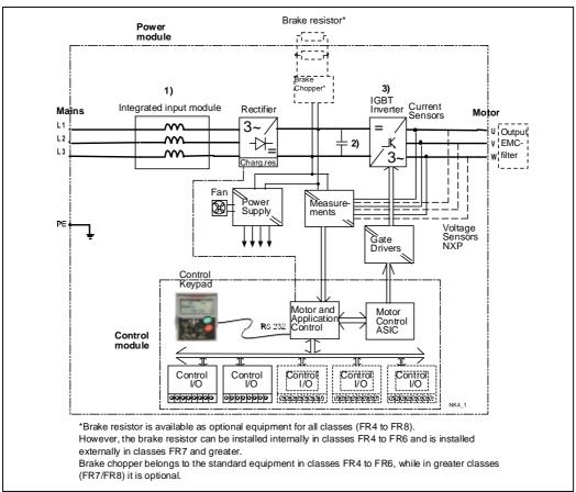
Figure 4-1. NX block diagram
