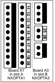
Figure 6-14. The I/O terminals of the two basic boards
