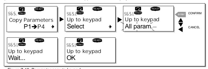
Figure 7-19. Parameter copy to keypad
