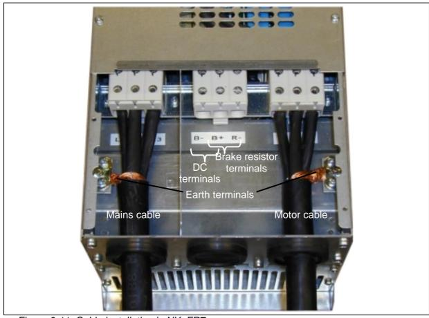
Figure 6-11. Cable installation in NX, FR7
