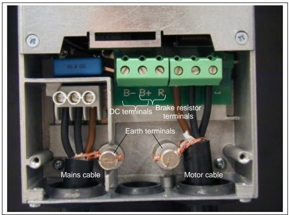
Figure 6-7. Cable installation in NX, FR5
