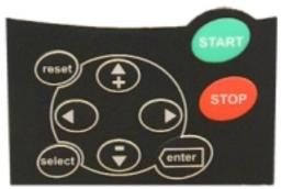
Figure 7-2. Keypad push-buttons
