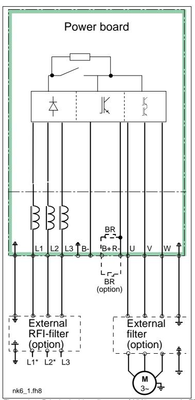
Figure 6-1. Principal wiring diagram of NX5 power unit, FR4 to FR6
