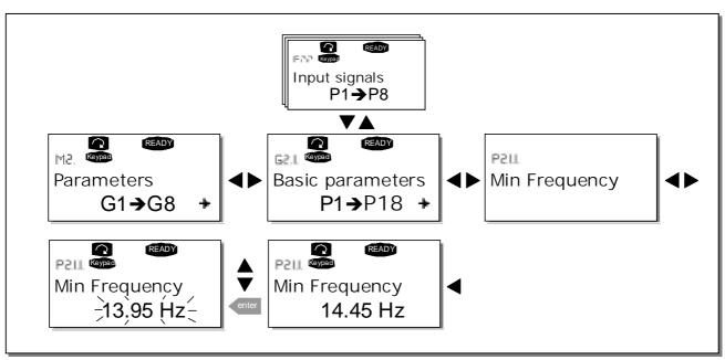
Figure 7-5. Parameter value change procedure
