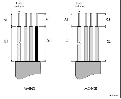
Figure 6-3. Stripping of cables
