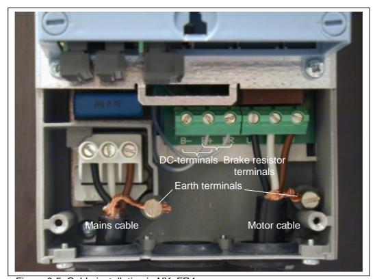
Figure 6-5. Cable installation in NX, FR4
