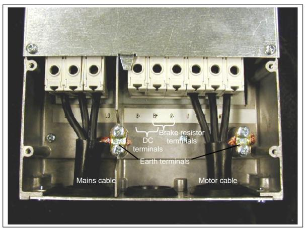
Figure 6-9. Cable installation in NX, FR6
