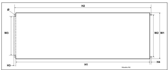
Figure 5-3. The opening needed for the collar installation, FR4 to FR6
