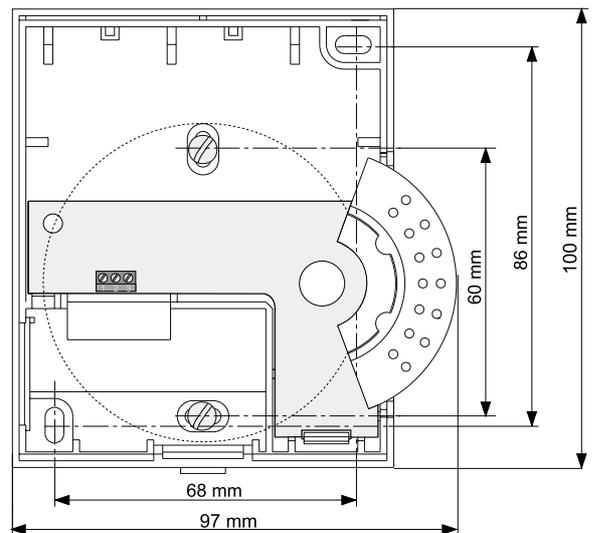
**Figure 2: Installation onto flush distribution box**
