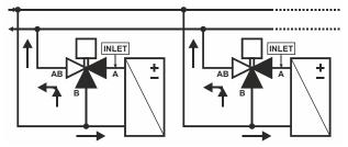
Fig. 5. Three-way mixing valve operation
