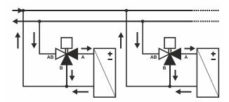
Fig. 6. Three-way diverting valve operation
