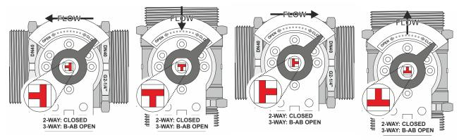
Fig. 7. Orientation of ball in valve / Linkage Positions for M6061/M7061
