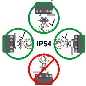
Fig. 8. Acceptable valve orientation
