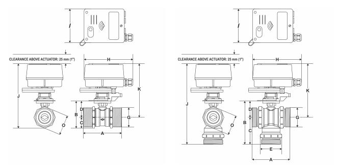
Fig. 2. M6061/M7061 + 2-way ball valve (see also Table 6)
