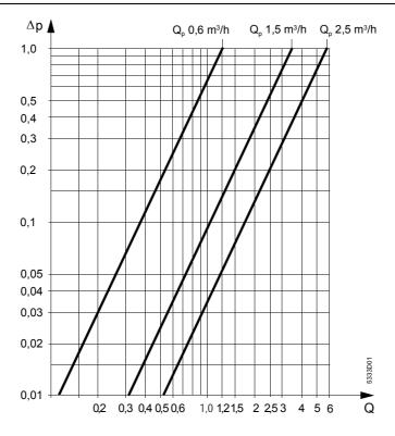
Pressure loss curve Pressure loss in bar
