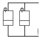
If no main flow sensor is installed, the controller adopts the measured value from the boiler sensor of the current lead boiler. Hence, the boiler sequence can be controlled with no need for using a main flow sensor.
