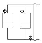
If a pressureless header is used, it is recommended to install a main return sensor.
