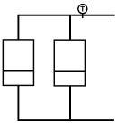
If no boiler sensor is installed, use of a main flow sensor is mandatory.
