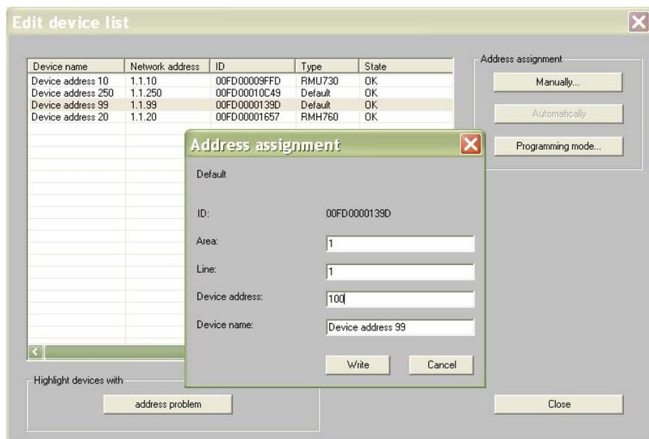
4. Enter a device address in the range 1...253 (excluding 150), and confirm by clicking the **Write** button.
