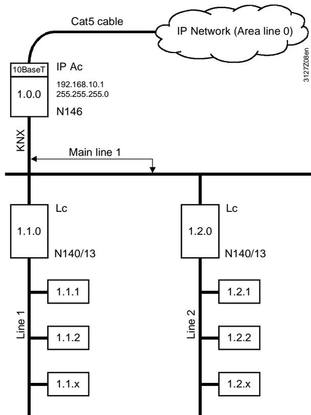
The IP router has a 10BaseT interface (Ethernet at 10 Mbit/s via Cat5 cable).
