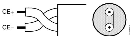
Unshielded bus cables are permitted for the KNX bus in conjunction with Synco devices. Shielded bus cables are recommended, however, if high interference is anticipated. For further details refer to data sheet N3127.
