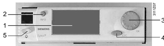
Plug-in type operator unit RMZ790
