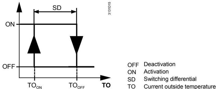
The relay contact closes when the current outside temperature falls below the level of Switch-off point minus switching differential. The relay contact will open again when the current outside temperature returns to a level above the switch-off point.
