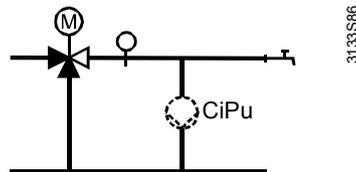
Consumer control always consists of mixing valve and consumer flow temperature sensor.
