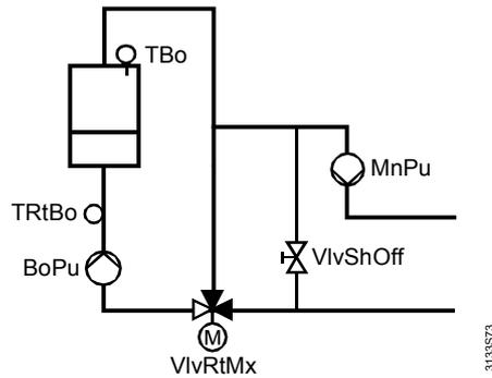
The 3-port mixing valve ensures both protective boiler startup and maintained boiler return temperature.
