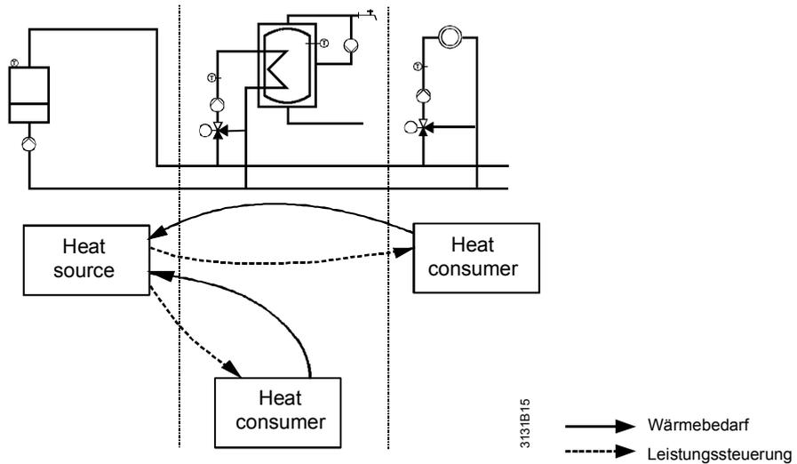
The temperature request for the current heat demand is calculated based on the flow temperature setpoint of the heating circuit (heating curve, subsection 9.5.2, and influences, subsection 9.5.3) plus an adjustable setpoint increase for the mixing valve.
