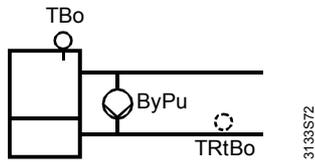
The bypass pump can be controlled either according to the acquired return temperature or, when there is no sensor, parallel to burner operation.
