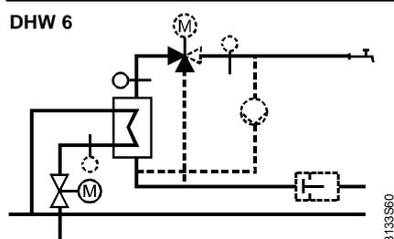
DHW heating takes place directly via the heat exchanger. Since there is no storage tank so that charging control cannot be provided, control is permanently enabled. The setpoint to be delivered by the heat source is made up of the current DHW setpoint plus the setpoint increase of the heat exchanger.
