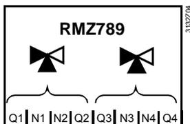
With the RMZ789 extension module, there are 4 mixing valve outputs available (for 2 mixing valves), where an RC unit can be activated.
