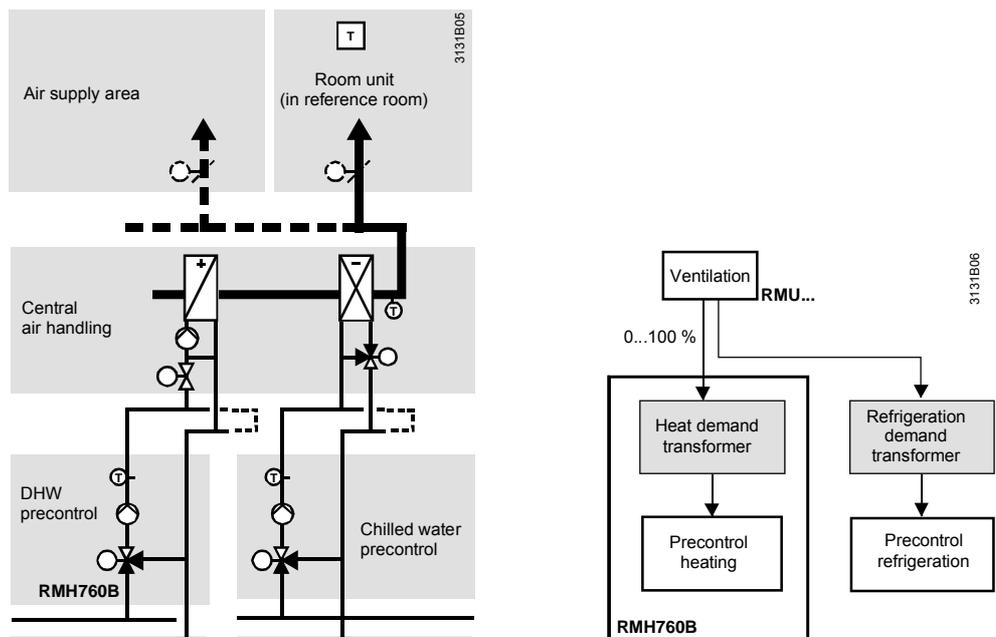
The heat demand transformers calculate a flow temperature setpoint based on the valve position of the air handling plant(s).
