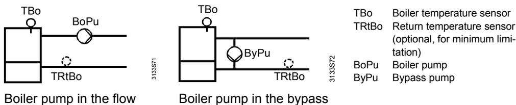
For plant types with boiler (H3-x and H4-x), a boiler pump is always configured. This boiler pump can also be operated parallel to the boiler, or it can be configured as a boiler bypass pump.
