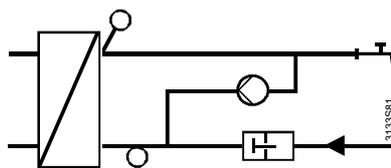
Use of a flow switch proves particularly advantageous in the case of smaller plants, such as single-family homes, but improves plant performance in all other cases as well. Fault status supervision is not possible since short-circuits and open-circuits are permitted states.
