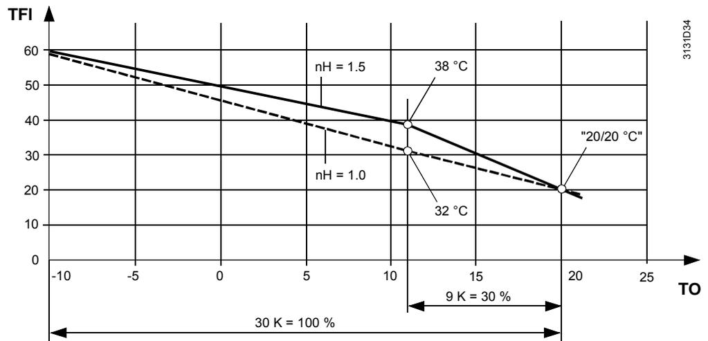
The lift at the point of inflection is dependent on the flow temperature setpoint and the radiator exponent.
