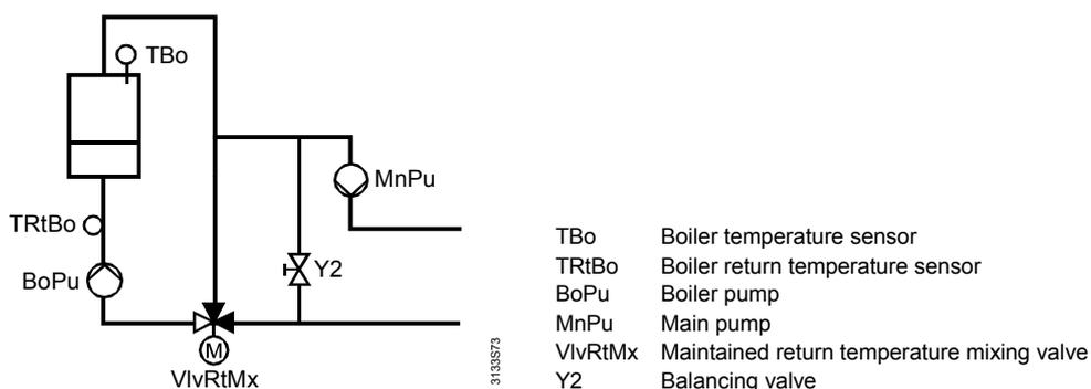
With plant types H4-x, the maintained boiler return temperature with 3-position mixing valve is already configured.
