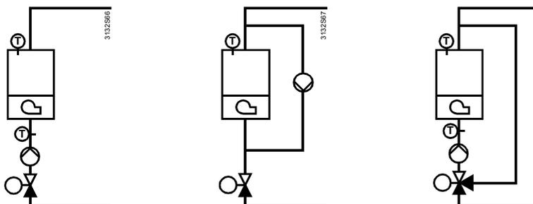
In most cases, the boiler can be hydraulically decoupled via a shutoff valve. In the case of plant with a mixing valve for minimum limitation for the return temperature, this function is performed by the mixing valve. If the boiler is not released, the mixing valve is driven to the fully closed position so that the boiler will be hydraulically decoupled from the plant.
