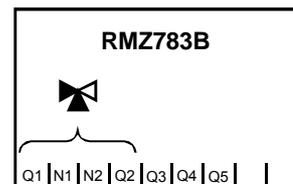
On the RMH760B basic unit and the RMZ782B and RMZ783B extension modules, terminal pair Q1/Q2 is used for activating an RC unit.
