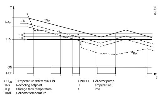
• The collector pump is switched on if the storage tank temperature lies at least 2 K above the recooling setpoint and above the collector temperature by temperature differential ON.
