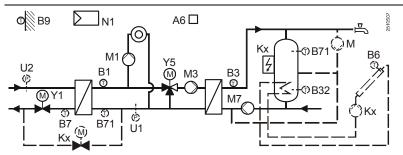
Two heat exchangers connected in series for heating circuit and d.h.w. heating. Instantaneous storage tank connected to the second heat exchanger, with mixing valve control for d.h.w.
