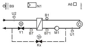
Heating circuit control without d.h.w. heating RVD140: Refill function optional
