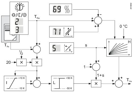
Generation of setpoint with room temperature-compensated control
