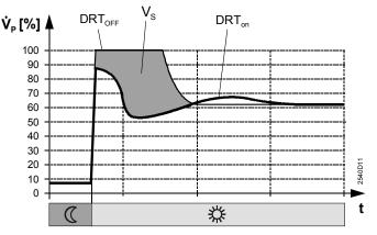
DRT<sub>ON</sub> Control with active limitation of the return temperature differential DRT<sub>OFF</sub> Control without limitation of the return temperature differential
