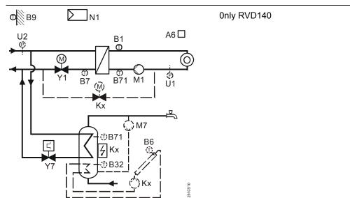
Heat exchanger for the heating circuit, d.h.w. heating via the district heat primary circuit, control of the d.h.w. temperature via an electrothermal actuator. Circulating pump, refill function, electric immersion heater and solar d.h.w. heating optional. For more detailed information, refer to section 14.5 "Plant type no. 6b". 3.2.8 Plant type no. 7
