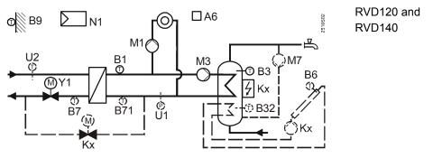
Heating circuit control with d.h.w. heating (storage tank). RVD140: Circulating pump, refill function, electric immersion heater and solar d.h.w. heating optional
