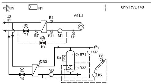
Separate heat exchangers for heating circuit and d.h.w. heating. Instantaneous storage tank connected to separate heat exchanger, d.h.w. charging with charging pump. Sensor B71 can be used as follows:
