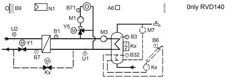
Heating circuit control with d.h.w. heating. Heating circuit with mixing valve, storage tank with charging pump.
