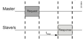
Maximum response time when reading: ...  $t_{resp}$  = 210 ms Maximum response time when writing:  $t_{resp}$  = 360 ms
