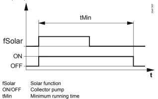
Special case: Frost protection Collector pump switch-off is delayed by the minimum running time after the frost protection limit is reached to flush the flow pipe between collector and storage tank with hot water.
