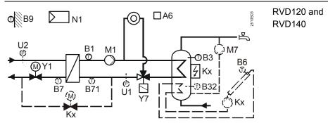
Heating circuit control with d.h.w. heating (storage tank). Circulating pump, refill function, electric immersion heater and solar d.h.w. heating optional.
